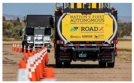
Figure 6. CDOT's Paint Truck with AMTA Vehicle.
